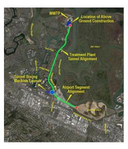
excavated diameter with a finished 12-foot inside diameter Fiberglass Reinforced Plastic (FRP) pipeline that extends from Bair Island to the WWTP. The project also includes shafts, drop facilities, ventilation, and odor control facilities. Once put into service, the pipeline will normally function to convey wastewater to the WWTP and will also be able to store peak flows for up to two days, mitigating the need for additional capacity upgrades at the plant.
